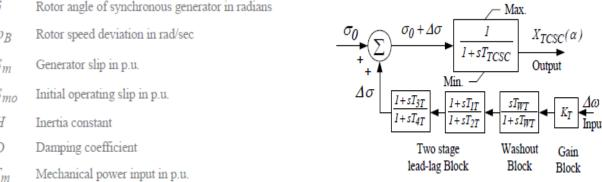
Fig: 2. Structure of TCSC-based controller
